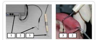
Figure 1: External view of the joule-metric device and clinical studies of periodontal tissue. (1, measurement unit; 2, passive electrode; 3, indicative electrode)
